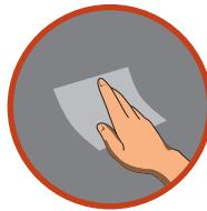
For fresh/ new surfaces, ensure the surface is clean and dry and free from all loose particles, chalk, grease, fungus and algae. Sand the surface with Emery Paper No. 80 and wipe clean.
