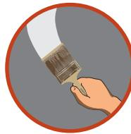
Apply the first coat of primer and allow it to dry for 6 – 8 hours.
